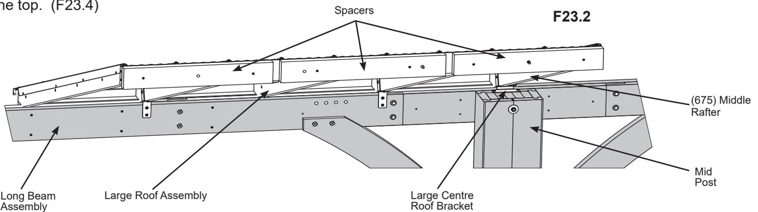
**One assembler to support roof panel(s) at all times until secure**
