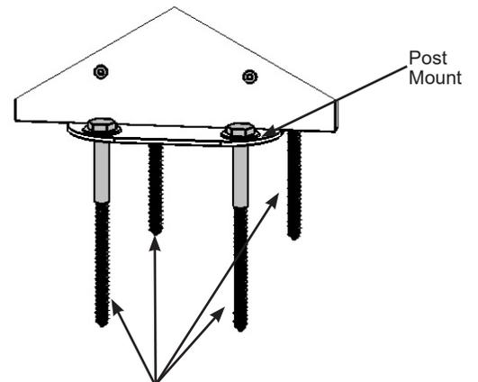
**Post Mounts have a 12.7 mm (1/2") diameter hole for anchoring hardware.**
