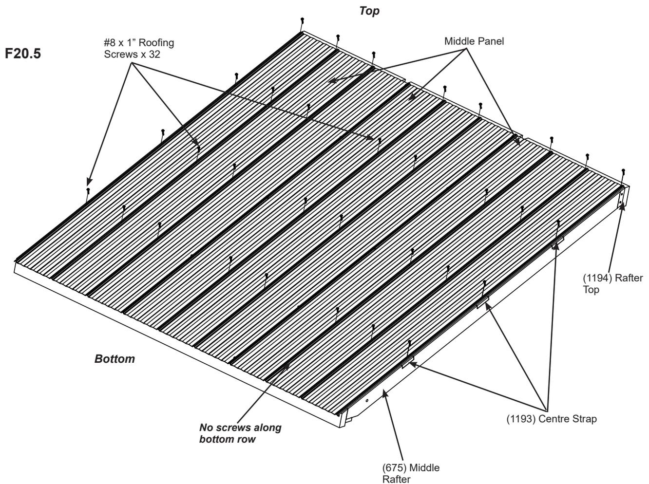
***DO NOT*** overtighten screws, could cause damage to roofing material
